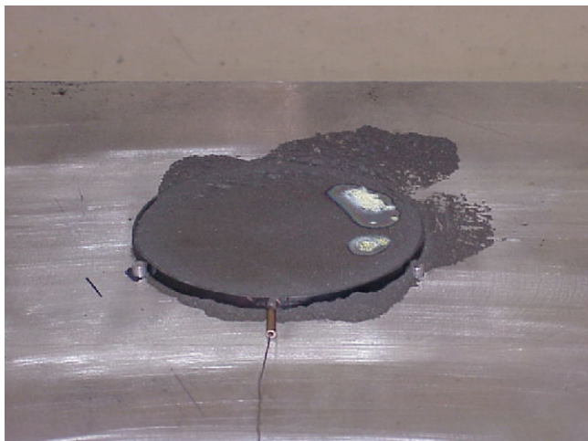
Fig. 3. View of the ignition of a 5 mm metallic dust layer during a self-ignition test.
